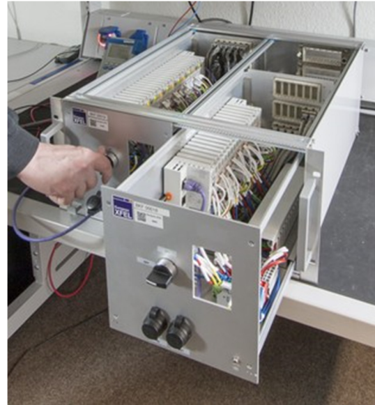
Figure 1: Image of the mechanical 19 inch frame with two PLC modules. The right module is only half-way inserted and allows to see the Harting Han series connector frame at the back.
