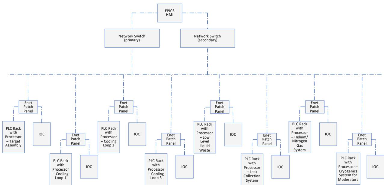
Figure 2: Distributed Control of Target Subsystem for STS.
