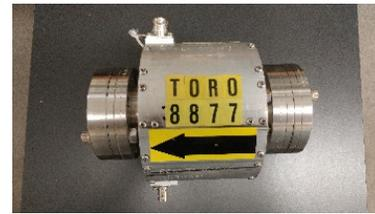
Figure 4: Toroid with two windings.
