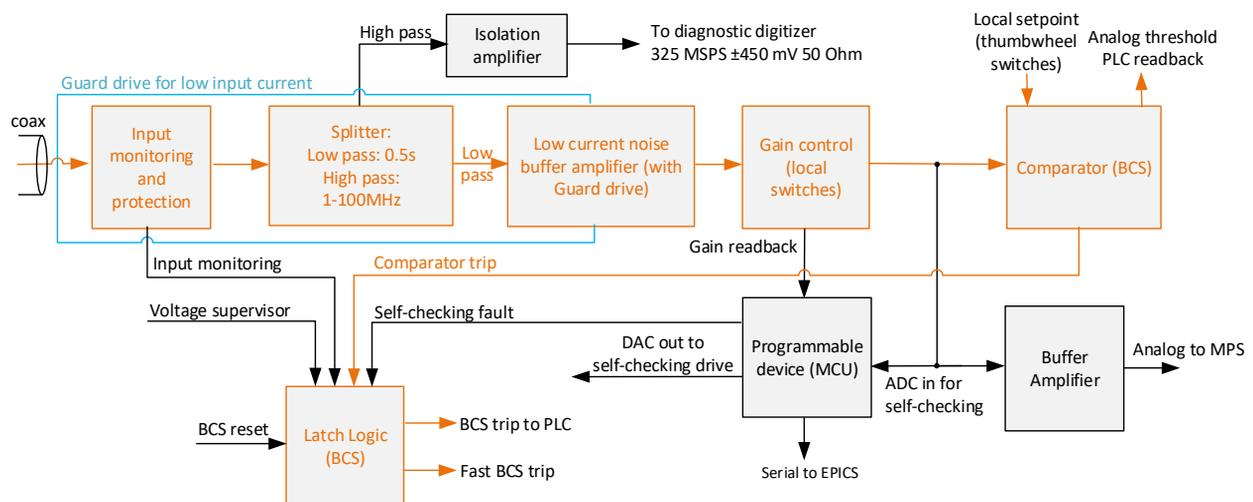
Figure 2: BLM electronics functional block diagram. The direct interlock path is highlighted.
