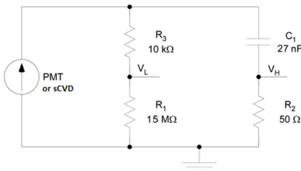
Figure 1: Input splitter and integrator circuit. Values shown for PBLM version of the electronics.
