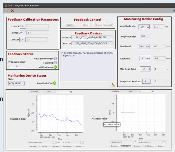
A Karabo scene to monitor and configure the XrayFeed device
