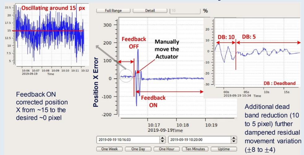
Effect of feed back on beam position stability using pop-in monitor as diagnostic device
