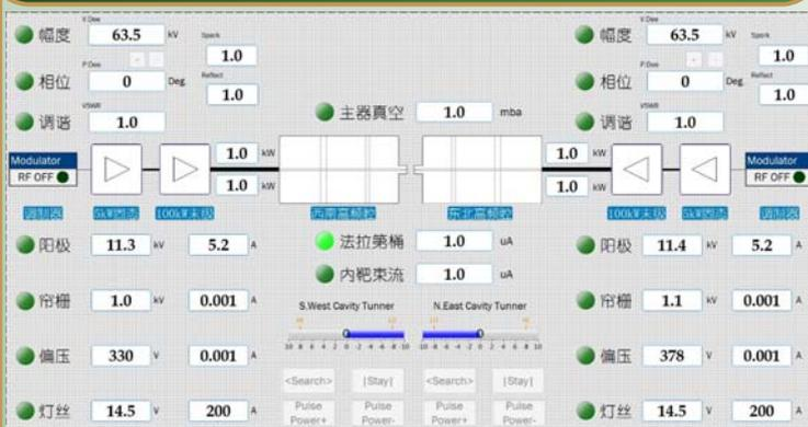
In the early stage, especially in the system development phase, this OPI interface was developed using Pyepics and PyQt frameworks. In the new OPI, we use the LED animation to display the switch status and use the text control to display the RF system information such as the Dee voltage, Driven amplitude, and phase, etc.
