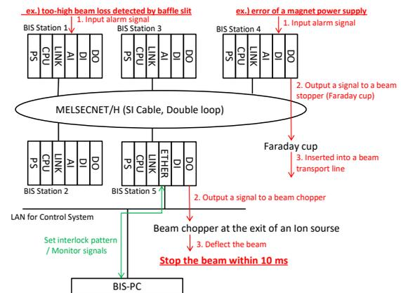
Figure 1: Example of the hardware configuration and process flow in BIS. The green line signifies communication via Ethernet.
