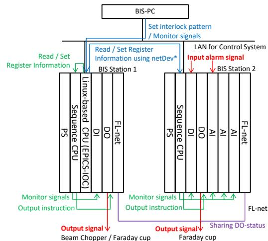
Figure 2: Hardware constitution and process flow in BIS2. Blue lines signify communication via Ethernet, green lines signify communication via PLC bus, and purple lines signify communication via FL-net.
