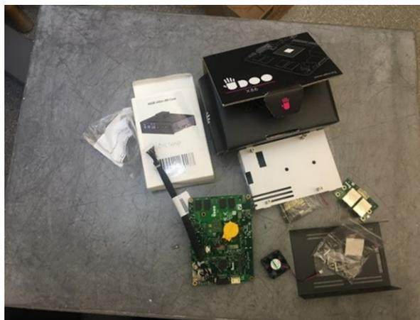
Figure 1: Unassembled hardware: UDOO Ultra board, two 1Gb Ethernet daughter card, metal case, cooling fan.
