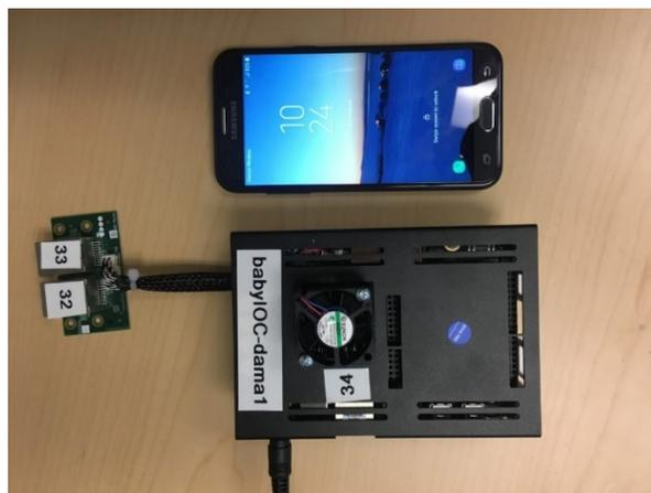
Figure 2: Assembled babyIOC.
