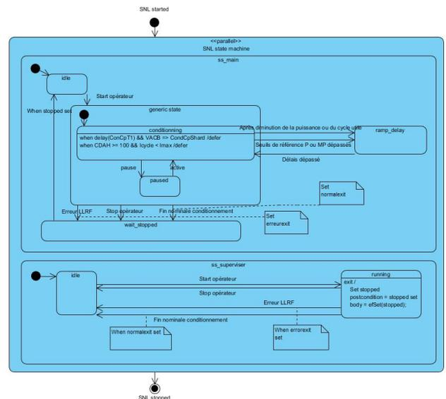
Figure 4: UML state diagram for coupler conditioning.
