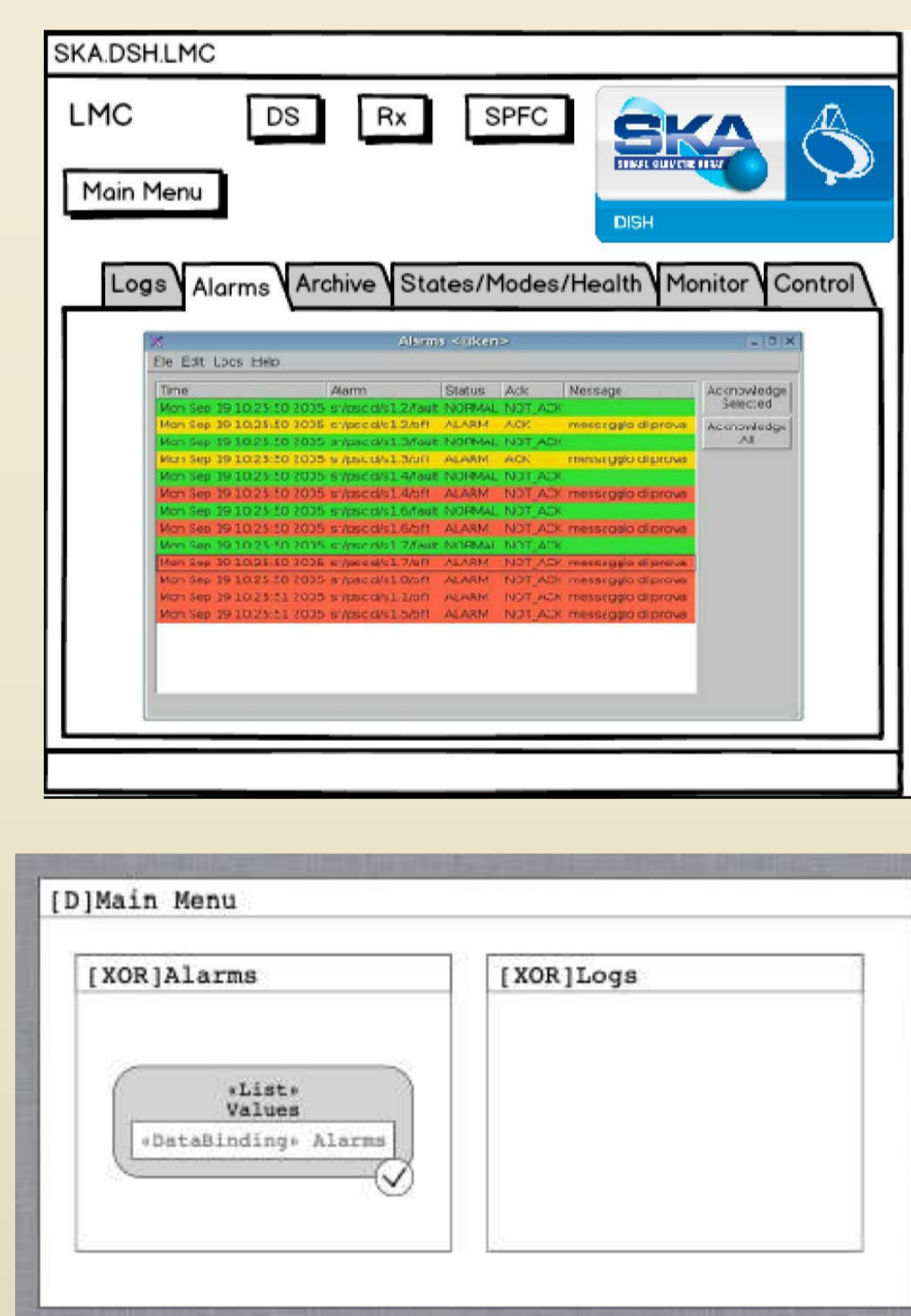
Figure 2 Sketch of DISH LMC engineering UI (top) and partial IFML conceptual model representing the UI part visible in the sketch (bottom)
